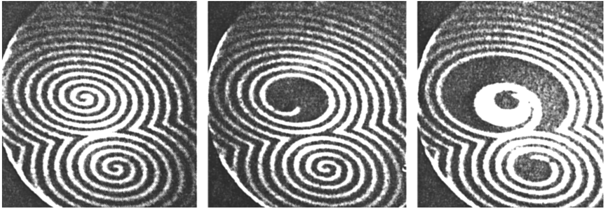
FIG. 2.10: Sequence of PEEM images at p_{\text{CO}} = 5.6 \times 10^{-5} mbar, p_{\text{O}_2} = 4.0 \times 10^{-4} mbar, and T = 483 K after a periodic forcing of the catalyst temperature; the section is 173 \times 173 \mu\text{m}^2 (after [6]).
